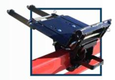
Standard large pad for draper heads (equivalent to previous model large pad).
