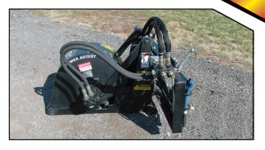
Hydraulic power adjust depth control — The patented power adjust depth control utilizes the bucket function of your skid steer to adjust the depth of cut of the planer. This simple to use method allows the operator to keep his hands on the controls at all times and gives precise control of the planing operation.
