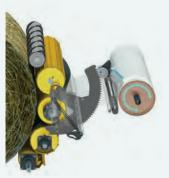
Net wrap is applied to the bale when the duckbill pivots into the chamber.
