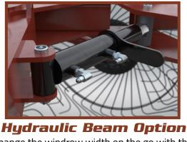
Change the windrow width on the go with the MCR's hydraulic beam option. These cylinders mount on the wheel beam and allow for total raking control.
