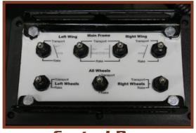
**Control Box** All controls are done from the tractor seat with convenient control box.
