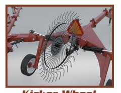
**Kicker Wheel** The MCR's hydraulic full size 55" kicker wheel prevents moisture from becoming trapped in hay at the center of the windrow
