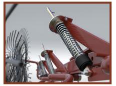
**Independent Suspension** Easily adjust spring tension for each wheel by simply removing a cotter pin. No tools necessary. Unique spring angle allows for consistent down pressure throughout wheel movement.
