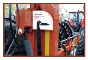
Wheel Angle Adjustment Quickly adjust wheel beam angle, allowing you to change for varied crop conditions.
