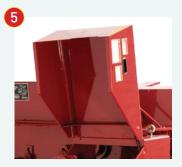
Steel shields give you easy access to key service points, like the gearbox and hydraformatic pump, the rotary feeding system chain,
