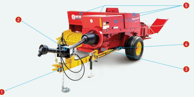
To accommodate large tractor drawbars without binding, all models feature a heavy-duty, easy-to-level tongue with a deep clevis (Hayliner 275 shown above). For added strength, the tongue is made of heavy-gauge steel with reinforced box construction, which pulls from the baler's axle to minimize towing stress.
