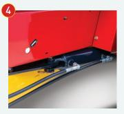
While mechanical tongue swing is standard, you can also use hydraulics to swing the baler into transport or working position quickly and easily. Hydraulic tongue swing is standard on the Hayliner 275 PLUS and available as a kit for the Hayliner 265 and Hayliner 275.
