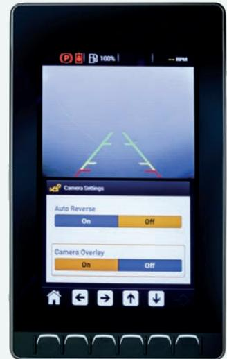
The integrated back-up camera on the HAWK display increases visibility to the rear of the loader, improving operator efficiency and safety. You can set the camera for "always on" or to engage only when shifting the loader into reverse gear.
