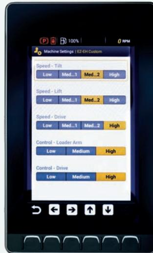
The HAWK display is easy to navigate and offers simple electro-hydraulic control settings. It's also customizable to an operator's preferences and lets you change settings for seasonal applications.
