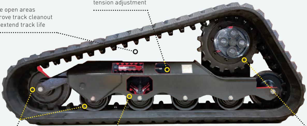
Lifetime sealed and lubricated rollers/idlers reduce maintenance costs
