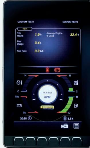
HAWK provides key operation data, including engine and performance information, RPM, fuel level, battery voltage, hydraulic oil temperature, engine temperature, and trip screen.
