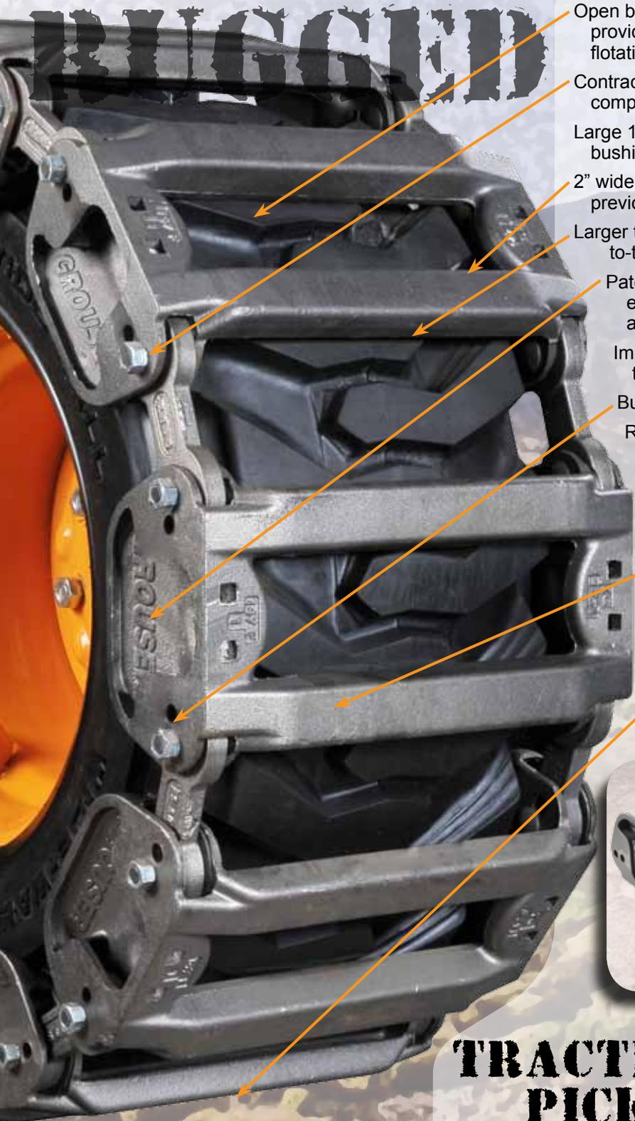
Open bar design utilizes the tire to provide maximum traction and flotation
