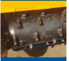
Fixed tooth forestry mulcher Suitable for managing wooded areas and provideing a chipped wood finish.
