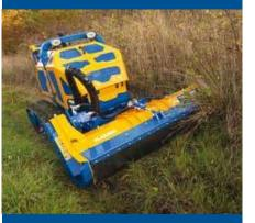
Hydraulic front hood Operational via controls with electronic interlock for safety dependent on rotor direction.
