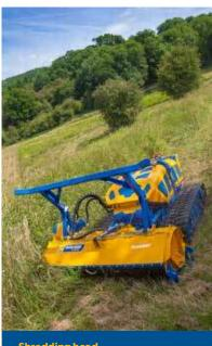
**Shredding head**Fitted as standard with 1650mm (5'5") shredding head and pushbar.
