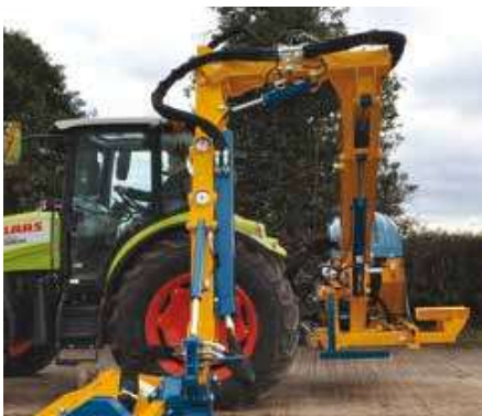
Telescopic 3rd arm on 6.0T and 6.5T models Gives increased flexibility.
