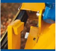
Auto swingover latch To operate fully extend second arm, allowing single operation from left to right.
