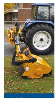
**Gravity breakout** For machine and operator safety.
