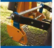
**Gravity breakout** To protect tractor and machine when cutting.
