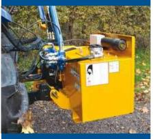
**Integral tank mainframe** Reduced weight makes the Raven compatible with smaller tractors.
