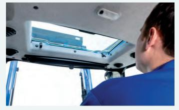
Optional **high-visibility panel** on all WORKMASTER<sup>TM</sup> cab models provides greater visibility, especially when working with a loader.
