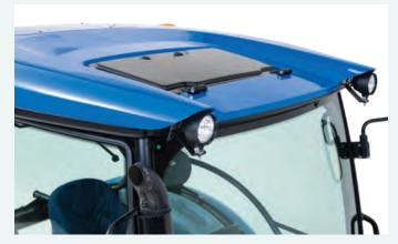
$\ensuremath{ \text{HVAC}}$  system features six roof vents and a blacked-out roof hatch that opens for ventilation.
