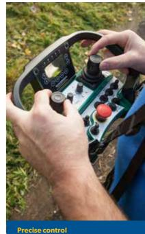
The remote control, operating all Flailbot functions has a range of 150m (492').
