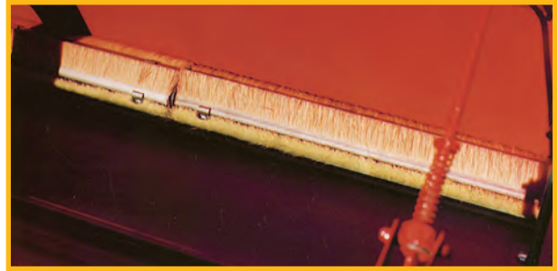
Brush Agitators - keep the seed flowing at a positive, accurate rate and provide instant shut-off the moment the seeder is stopped; prevents seeding "skips" and bunching of seeds.
