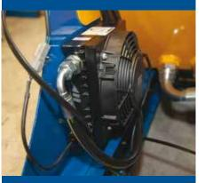
Optional oil cooler Can be fitted in rear panel.
