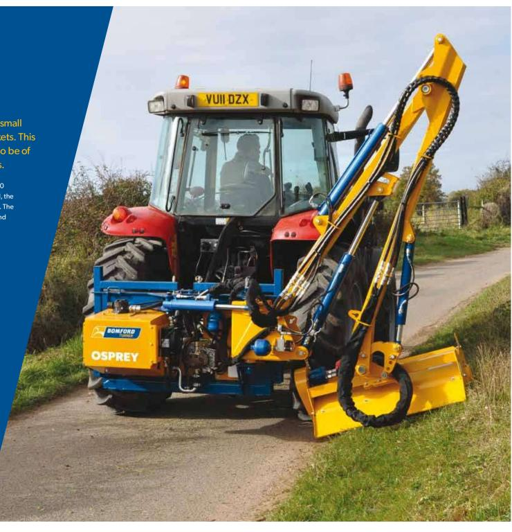
Hydraulic slew & breakout 110° of slew and hydraulic breakout makes the Osprey very adaptable.
